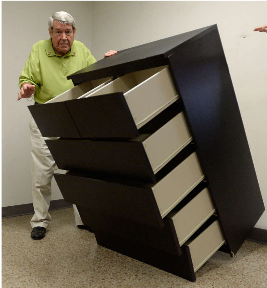
Bobby Puett , president of Diversified Testing Laboratories, watches as IKEA's MALM six-drawer dresser falls over during a test in Burlington, N.C. SARA D. DAVIS / For The Inquirer
